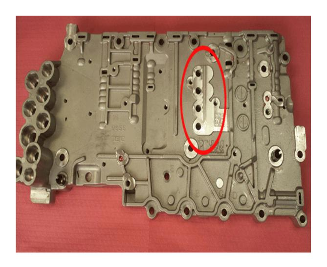
The oil passage holes that feed the center support and Low and Reverse Clutch and 2-6 Clutch contained within the center support vary location by transmission and corresponding upper valve body. The ISS and OSS mounting locations also vary by transmission. The incorrect valve body does not properly locate the oil feed holes and speed sensors.
