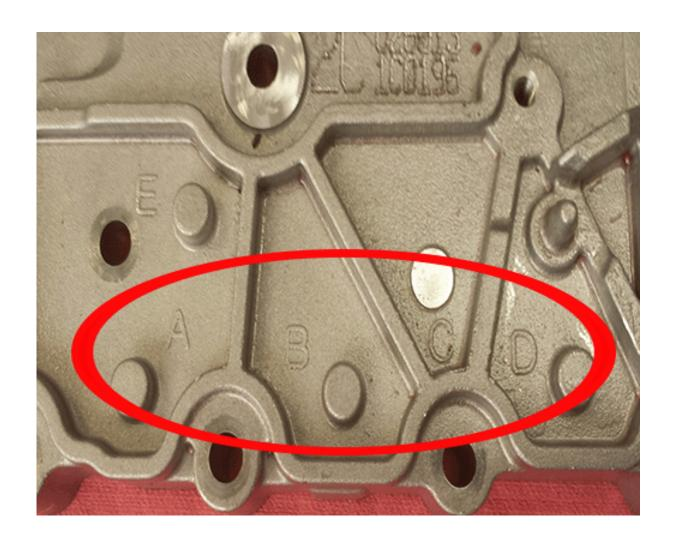
The post corresponding to the correct RPO will be milled off. In this case the "C" post is milled indicating that this is an MYC upper valve body. A milled "A" post indicates MYA, a milled "B" indicates MYB, a milled "C" indicates MYC and a milled "D" indicates MYD.
