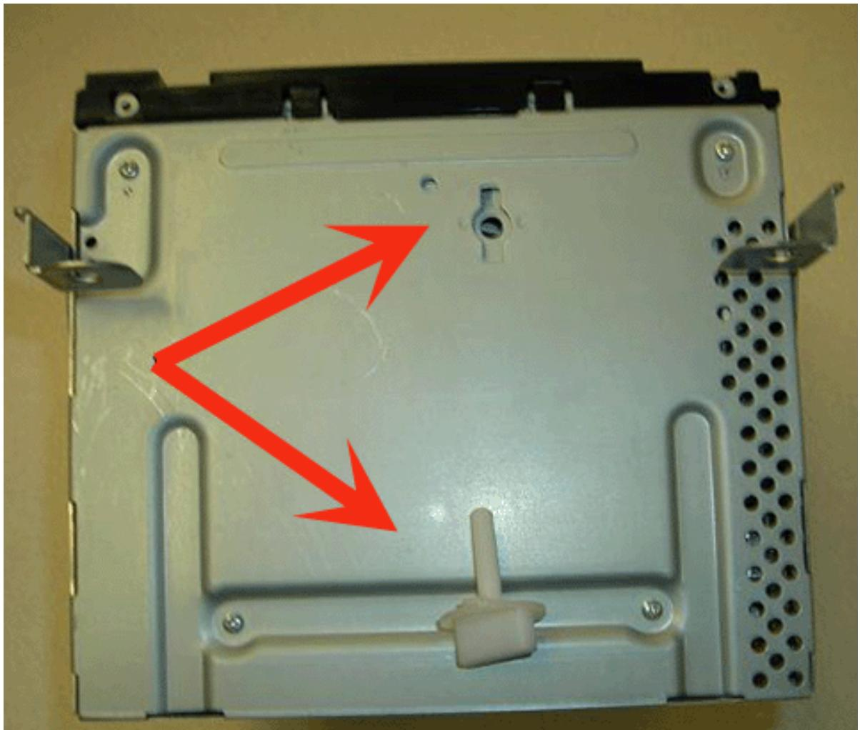
Remove the shipping pin from the bottom of the CD changer prior to installing into the vehicle. This item is called out by an arrow in the first picture below. The second picture shows the shipping plug that has already been removed from the CD changer.
