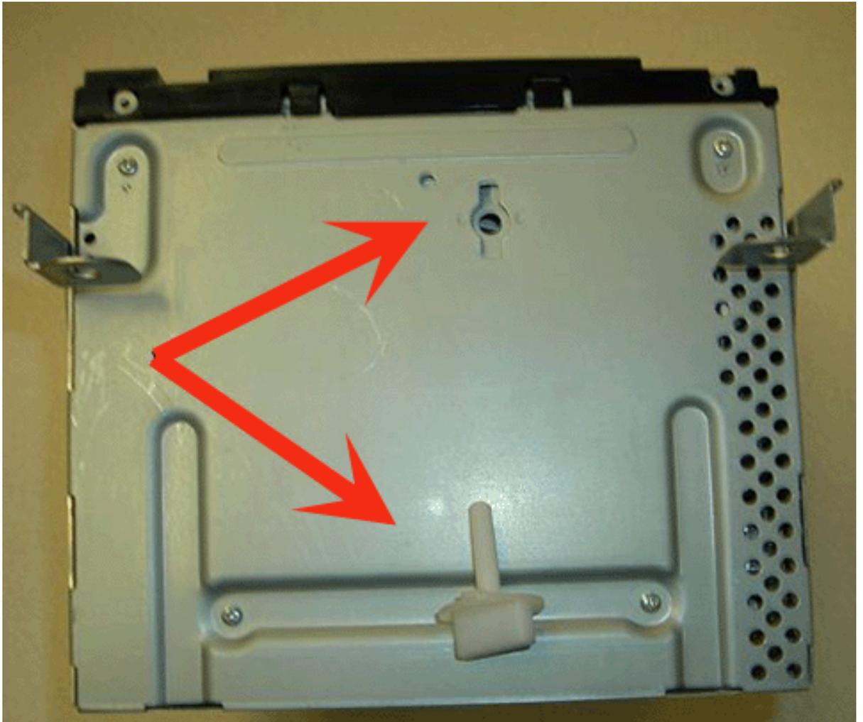
Remove the shipping pin from the bottom of the CD changer prior to installing into the vehicle. This item is called out by an arrow in the first picture below. The second picture shows the shipping plug that has already been removed from the CD changer.
