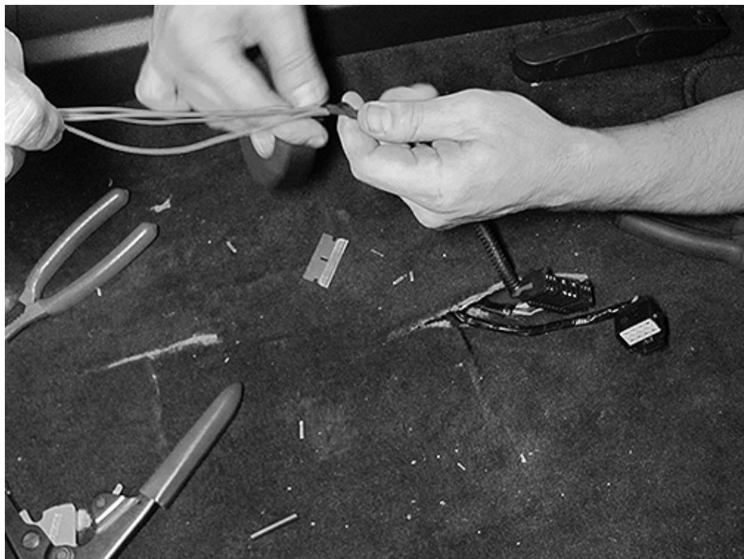
14. Wrap woven polyester electrical tape (PET) or equivalent anti-abrasion tape around the spliced section of the harness.
