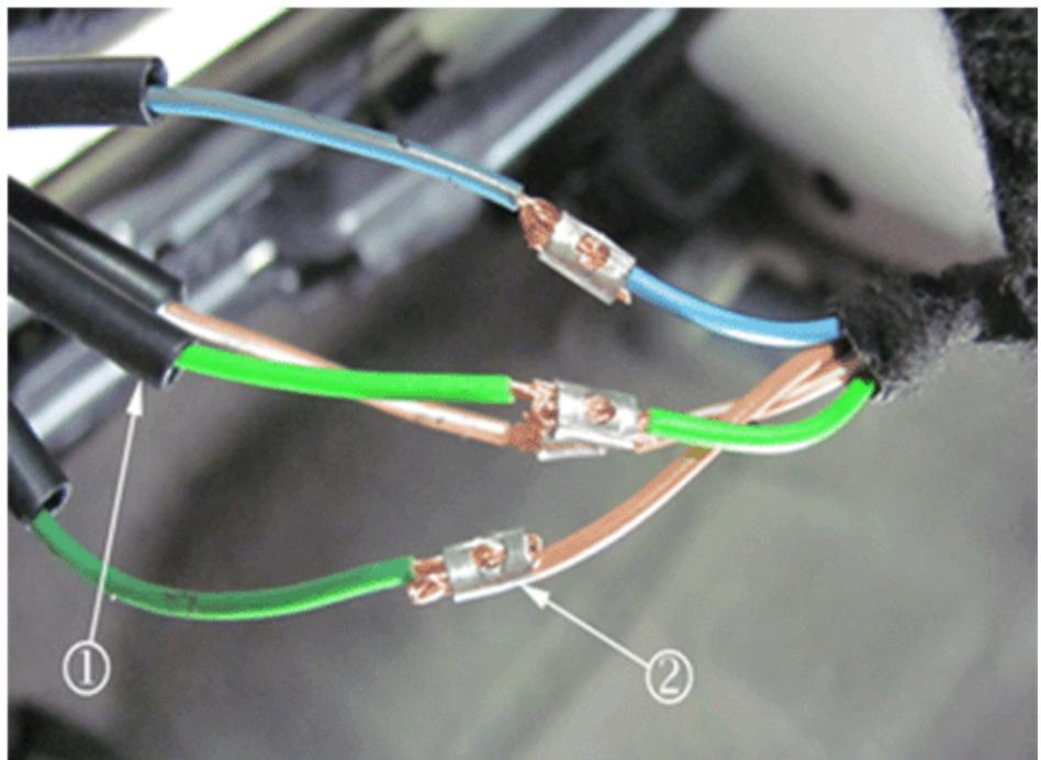
5. Add one approximate 38 mm (1.5 in) section of heat shrink tube to each of the four wires (1).
