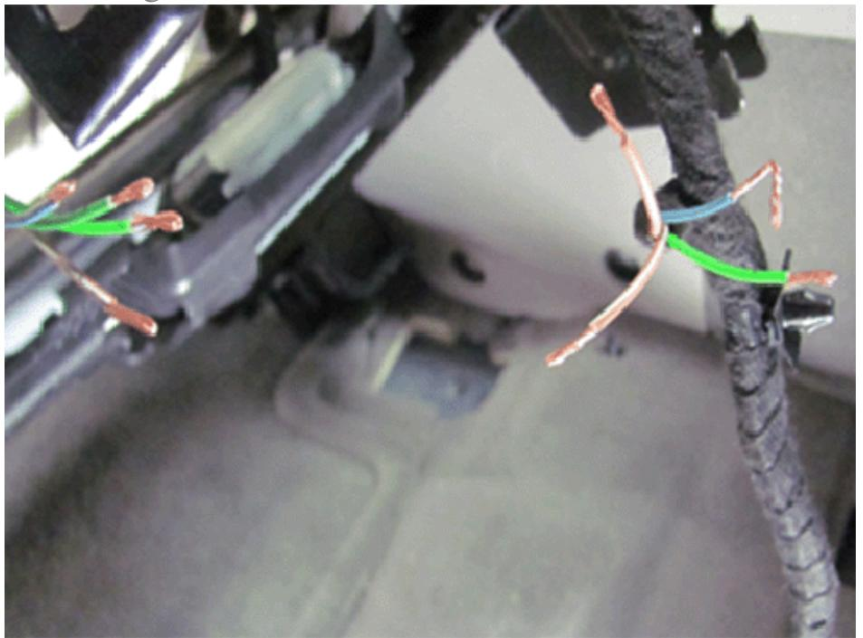
4. Strip off approximately 13 mm (1/2 in) of insulation from the wiring ends. Fold the wires.
