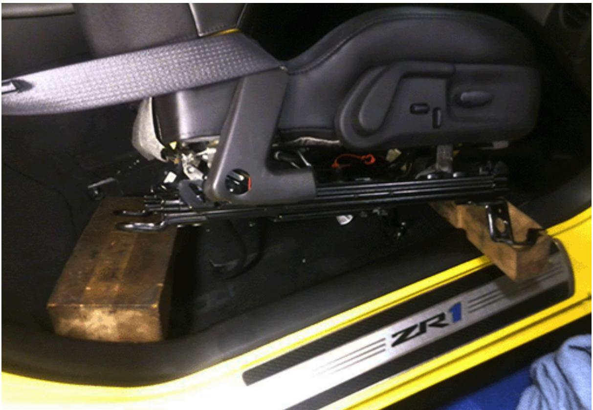
1. Using wood blocks or similar material, tilt and support the seat in the vehicle as shown.
