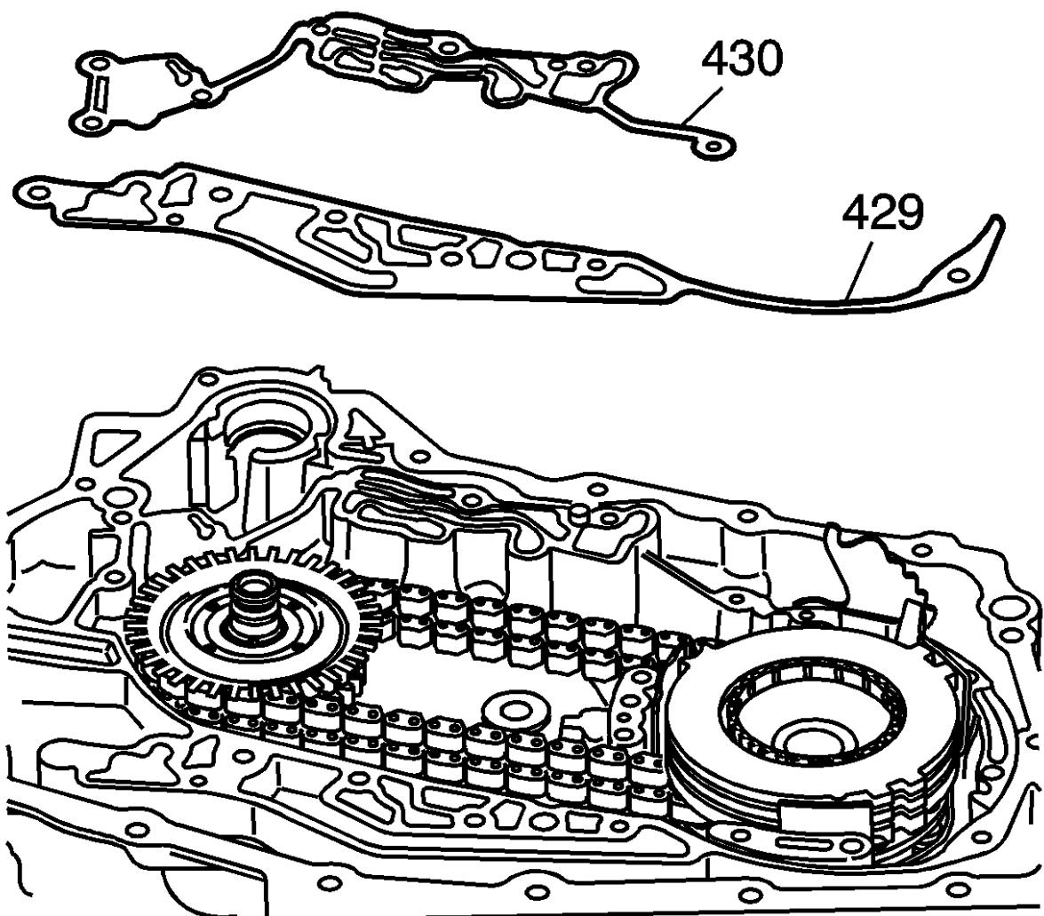
To correct this condition, replace the case cover (channel plate) gaskets (429 and 430). Refer to Unit Repair publication in SI of the appropriate vehicle being serviced.
