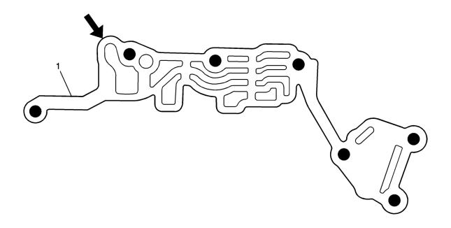
Visual inspection of the upper gasket (1) will reveal damage at the referenced area.
