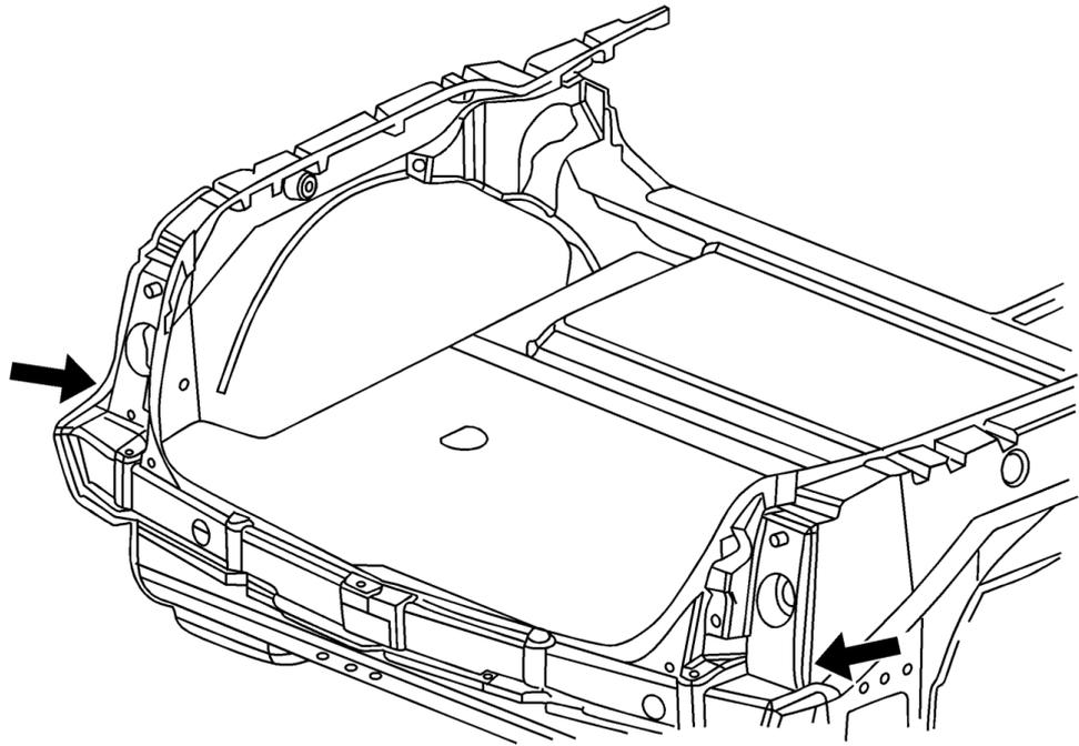
There are a number of panels that are bonded together in this area. If water entry is traced to this area, remove the rear tail lamp on the affected side to help gain access. Use Kent Seam Sealer, P/N P10200, to seal the affected joint. Refer to the illustration above.
