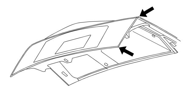
Seal the area of the rear compartment lid inner and outer panels at the outer most vertical seam (between arrows – either side). The seam is on the inside of the rear compartment lid. Refer to the illustration above. Use Kent Seam Sealer, P/N P10200, to seal the seam for best appearance.
