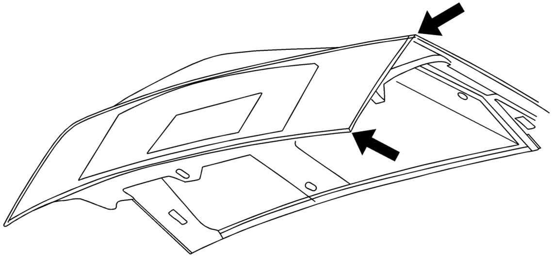
Seal the area of the rear compartment lid inner and outer panels at the outer most vertical seam (between arrows – either side). The seam is on the inside of the rear compartment lid. Refer to the illustration above. Use Kent Seam Sealer, P/N P10200, to seal the seam for best appearance.
