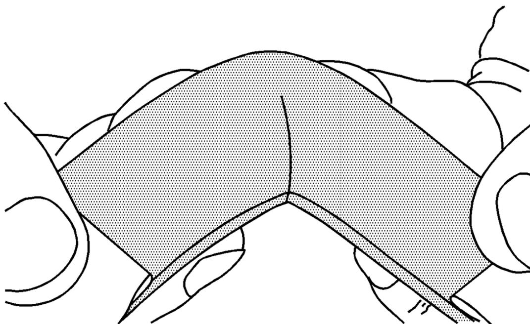
3. Pull back the adhesive paper protector near the notches and bond the notch together with weatherstrip adhesive
