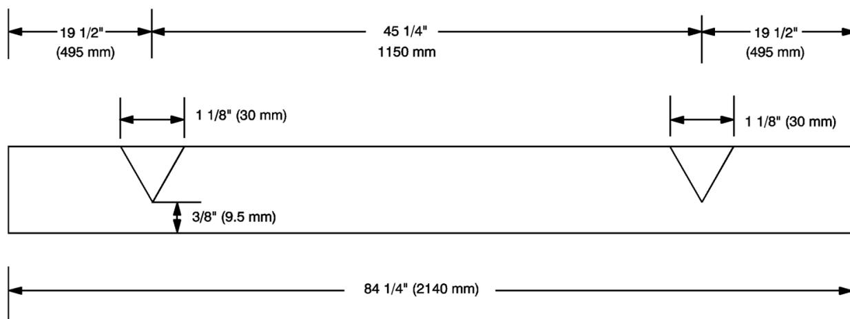
2. Cut the Kent Automotive Adhesive Shim Stock, P/N 46475, to the dimensions shown in the illustration.
