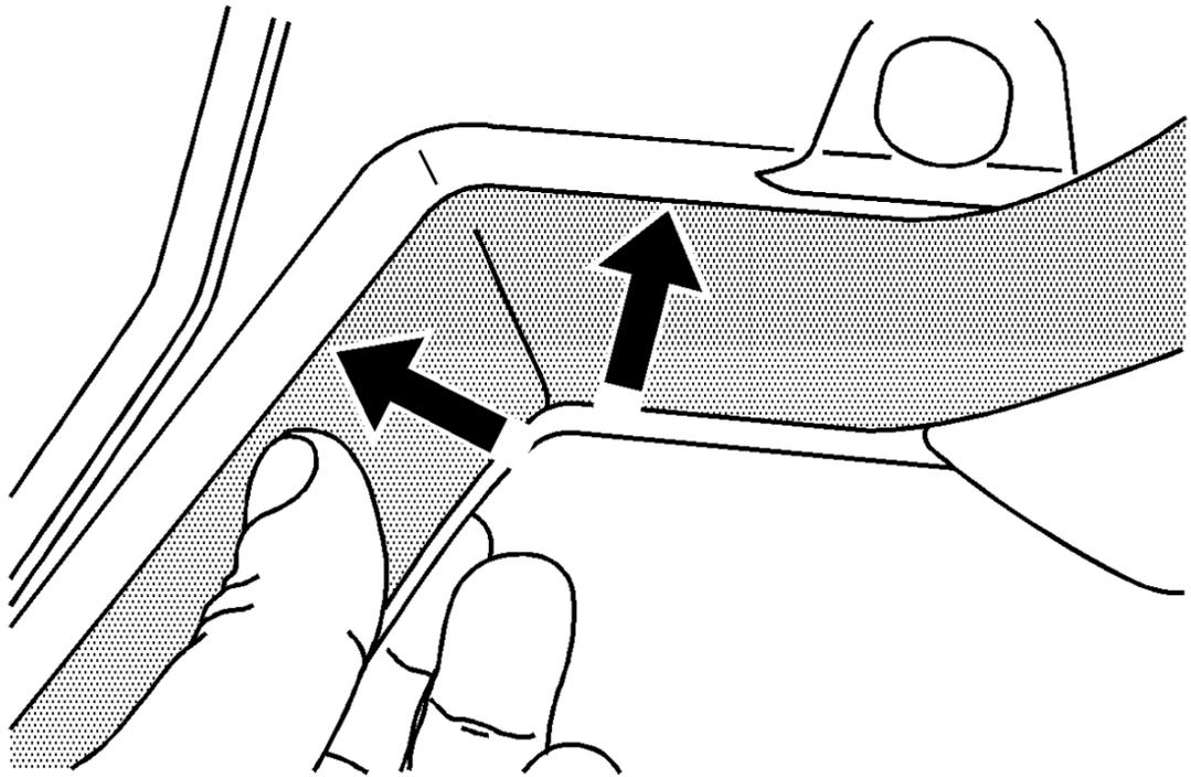
4. Insert the foam at each corner. Be sure to place it against the deck lid inner, following the ridge.
