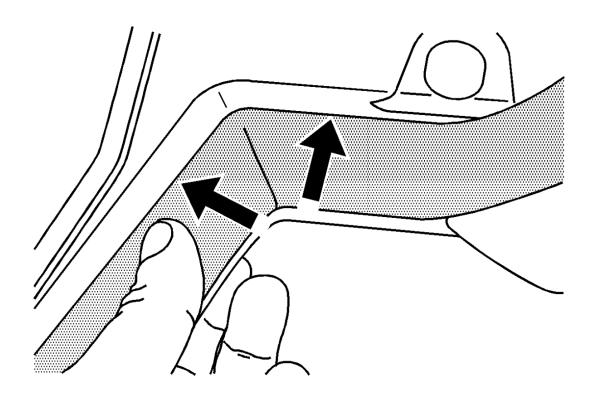
4. Insert the foam at each corner. Be sure to place it against the deck lid inner, following the ridge.
