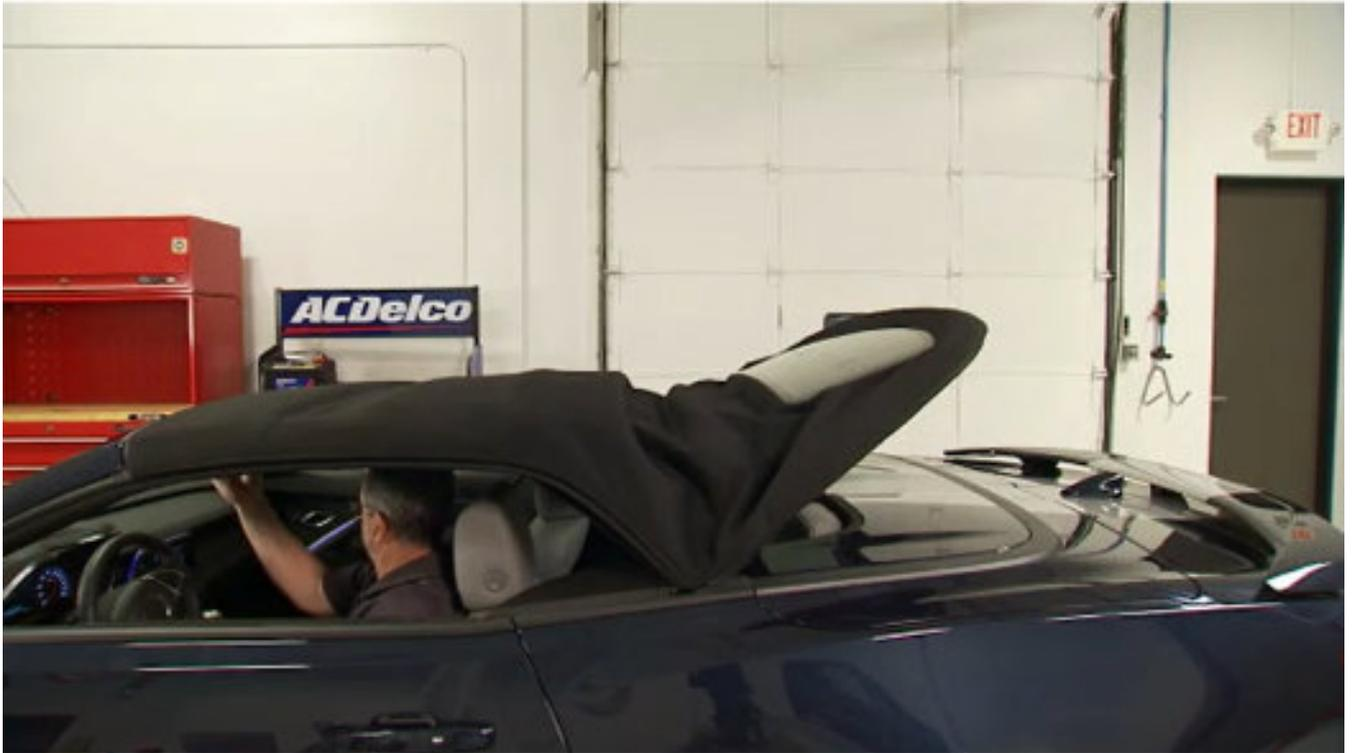
On a correctly working car, the stowage compartment lid must close completely before the tension bow is commanded down. Because the steps or phases must be completed in order, the technician must go to the point where the failure occurs, and then go back one step to look at the scan tool data.
