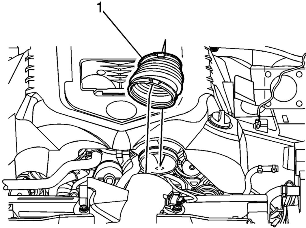
2) Tighten the 526, 852, and 853 supercharger inlet duct clamps to 2.5 NM (20 lb-in).
