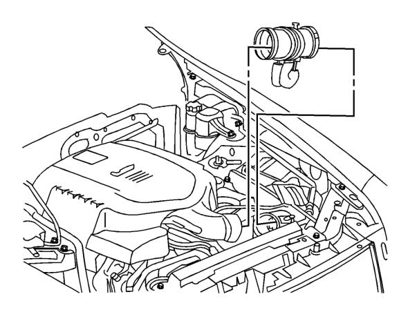
2) Tighten the 526, 852, and 853 supercharger inlet duct clamps to 2.5 NM (20 lb-in).
