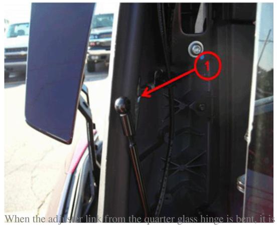
outboard. Refer to call out 1 in the illustration above. Bend the link back inboard until it will just touch the inside surface of the weatherstrip. When in the right position it could be forced passed the weather strip with minimal effort.
