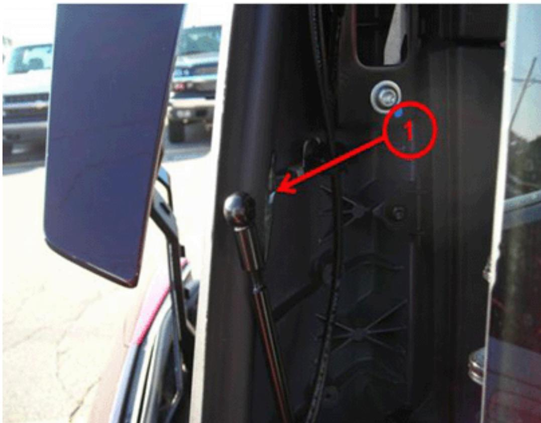
When the adjuster link from the quarter glass hinge is bent, it is outboard. Refer to call out 1 in the illustration above. Bend the link back inboard until it will just touch the inside surface of the weatherstrip. When in the right position it could be forced passed the weather strip with minimal effort.
