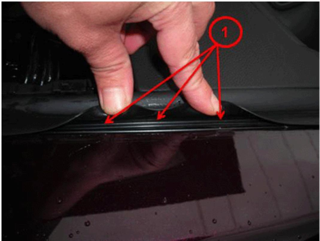
Push the quarter belt seal out of the outboard side of the retainer. Apply weatherstrip adhesive on the weatherstrip where it engages the retainer lip, see call out 1 in the illustration above. Reinstall the weatherstrip into the retainer. Lower the roof to hold the weatherstrip in place until the adhesive cures.
