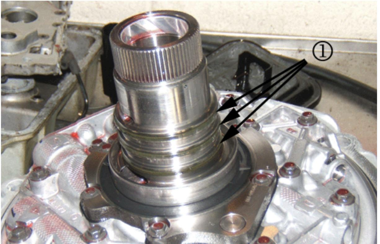
Inspect the fluid seal rings. Transmissions in 2006, 2007, 2008 and early build 2009 models used a 1- piece design seal ring in production. Starting December 2008, a 2-piece seal ring design was implemented. The 1-piece seal ring design may cause a harsh 2-3 shift due to leakage. This is typically a low mileage issue. If the seal rings are a 1-piece design they should be replaced with new 1-piece design seal rings. It is not necessary to replace the pump cover.
