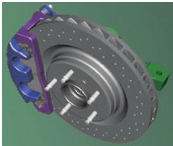
If required, these brake rotors can be machined on a lathe in a similar manner to standard rotors.
