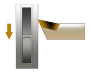
Using SI procedures, apply a non-directional finish to the rotor surface after machining by using a sanding block and 150-grit aluminum oxide sandpaper.
