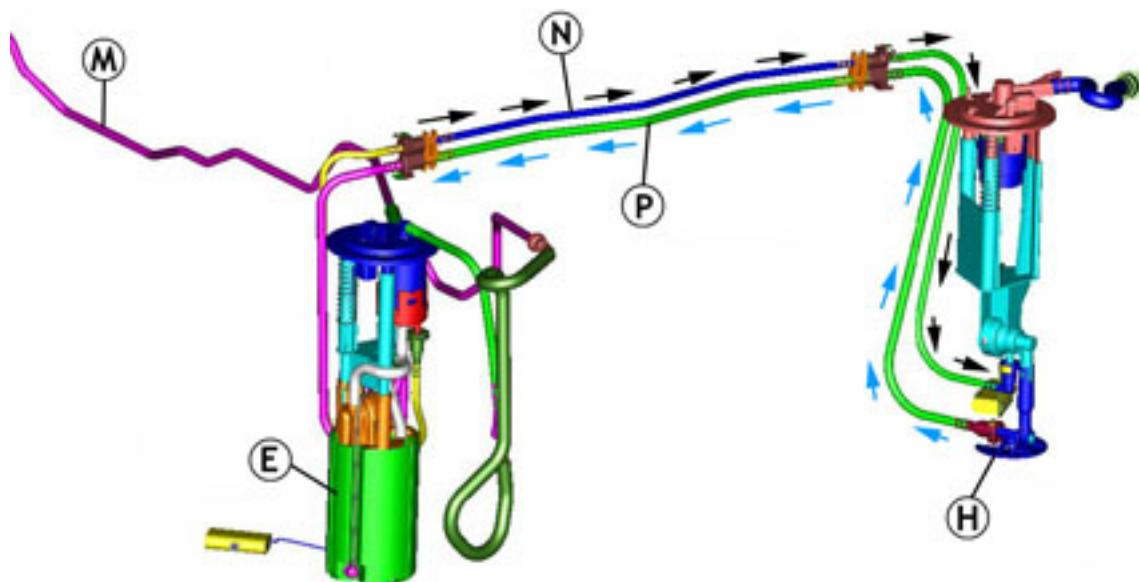
**TIP:** The pressure regulator is in the fuel tank, not on the fuel rail on the engine. This type of fuel system is called returnless, or demand. This means that excess
