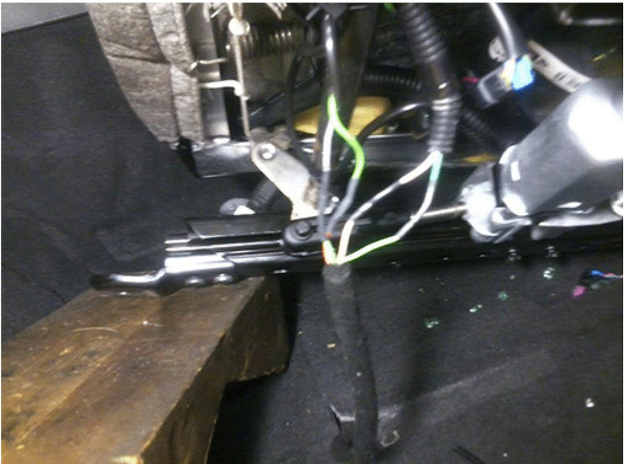
1. Center the heat shrink tube over all four splices and shrink/seal the heat shrink tube securely over the splice crimp and insulated wires.
