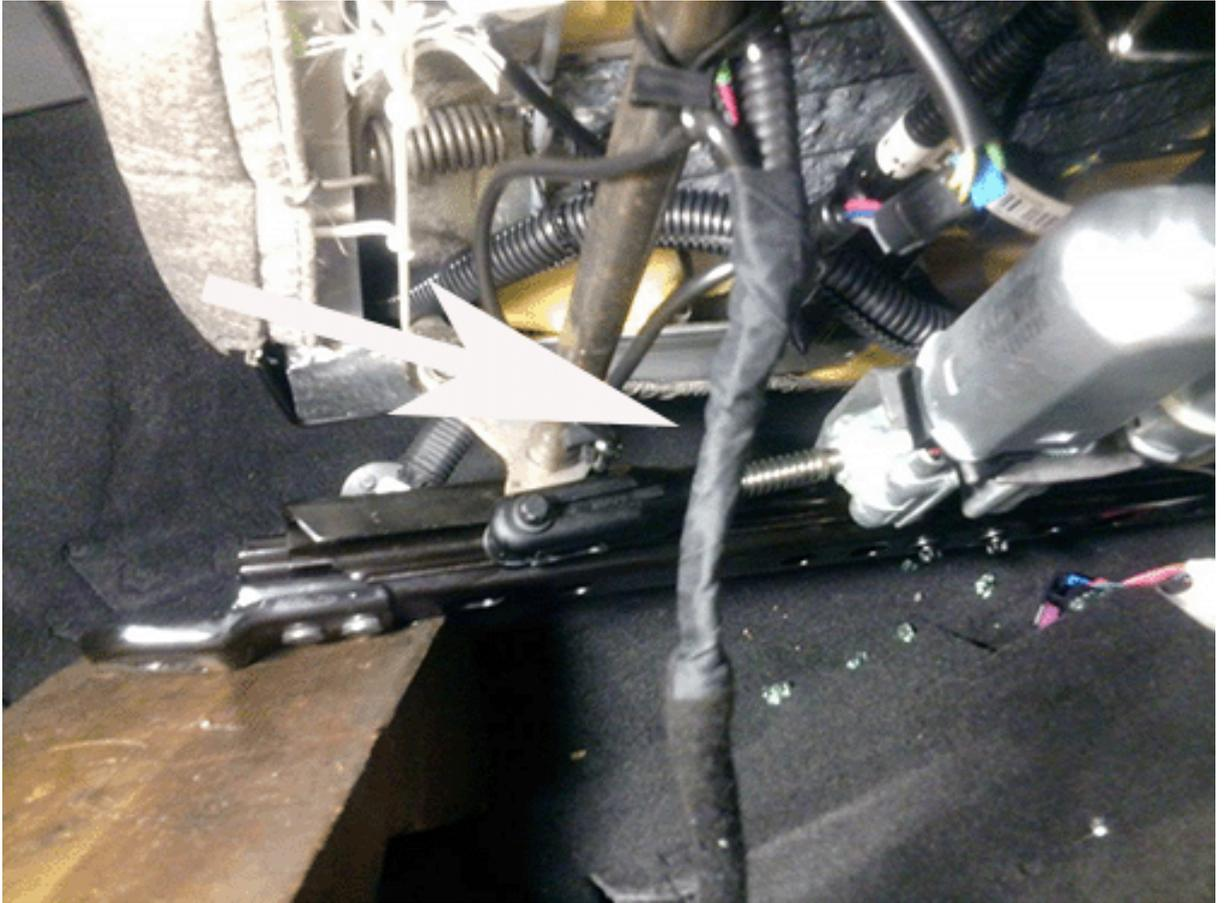
1. Wrap woven polyester electrical tape (PET) or equivalent anti-abrasion tape around the spliced section of both wires. Continue to wrap the harness as shown.
