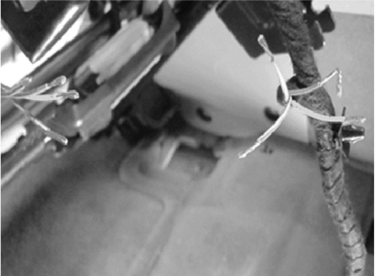
1. Strip off approximately 13 mm (1/2 in) of insulation from the wiring ends. Fold the wires.
