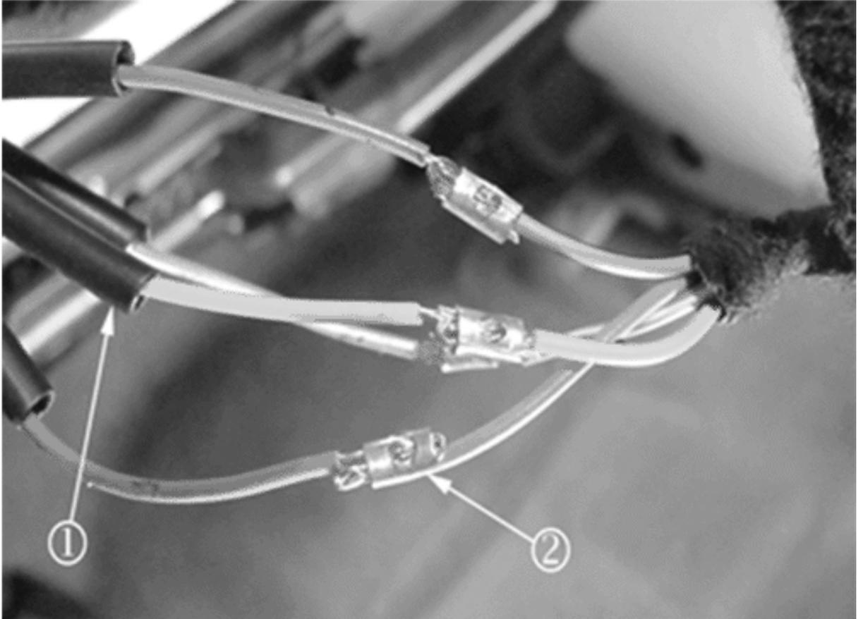
1. Add one approximate 38 mm (1.5 in) section of heat shrink tube to each of the four wires (1).
