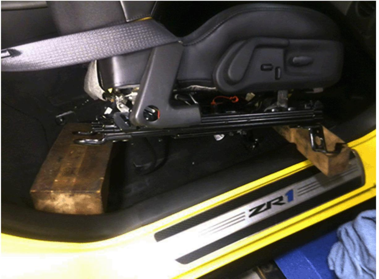
**Important:** Use care to not damage the sill plate or interior trim. Cover the area with a heavy shop cloth, masking tape or similar protective measures.
