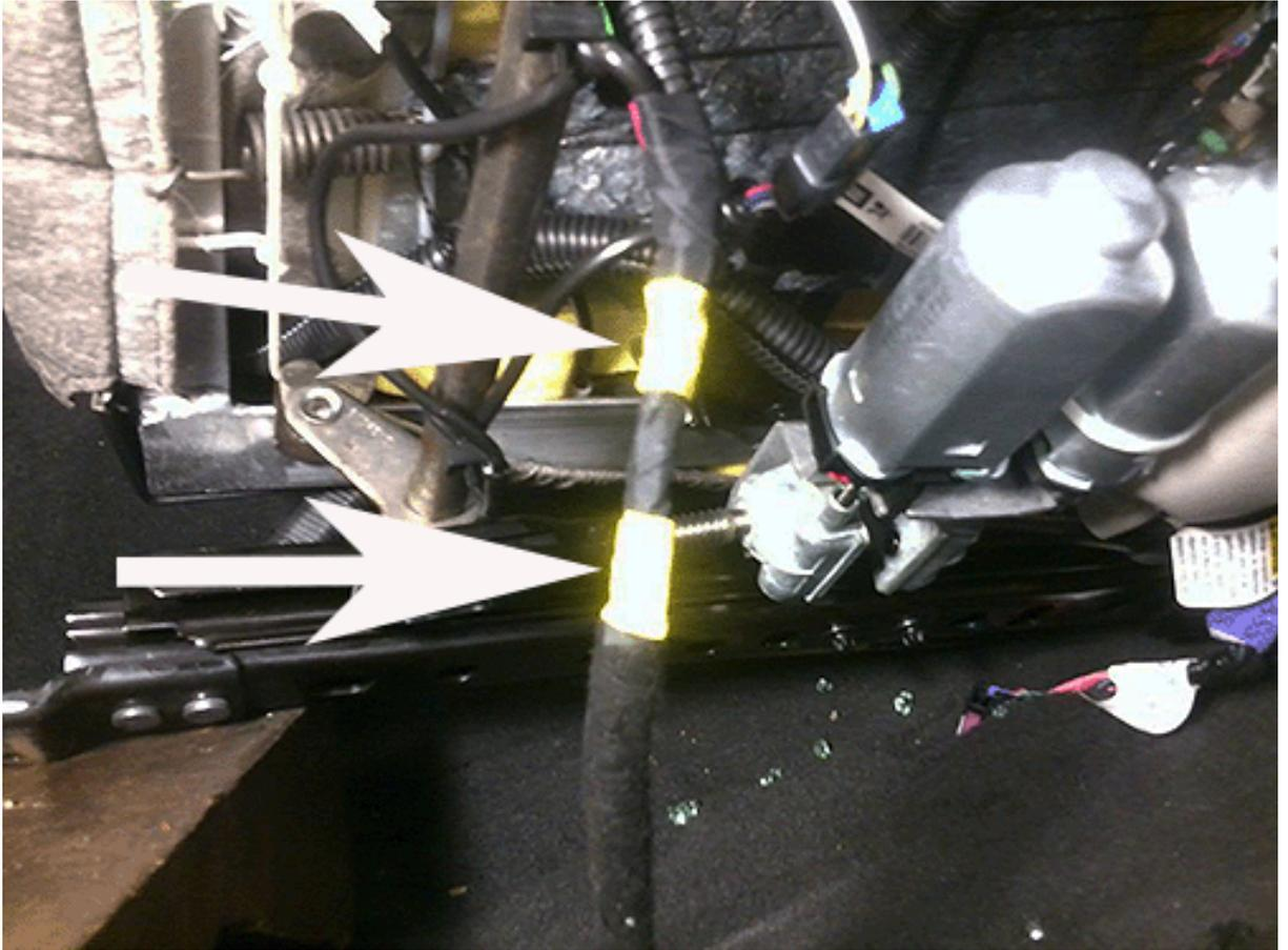
1. Wrap two sections of yellow electrical tape over the polyester electrical tape on both sides of the splice.
