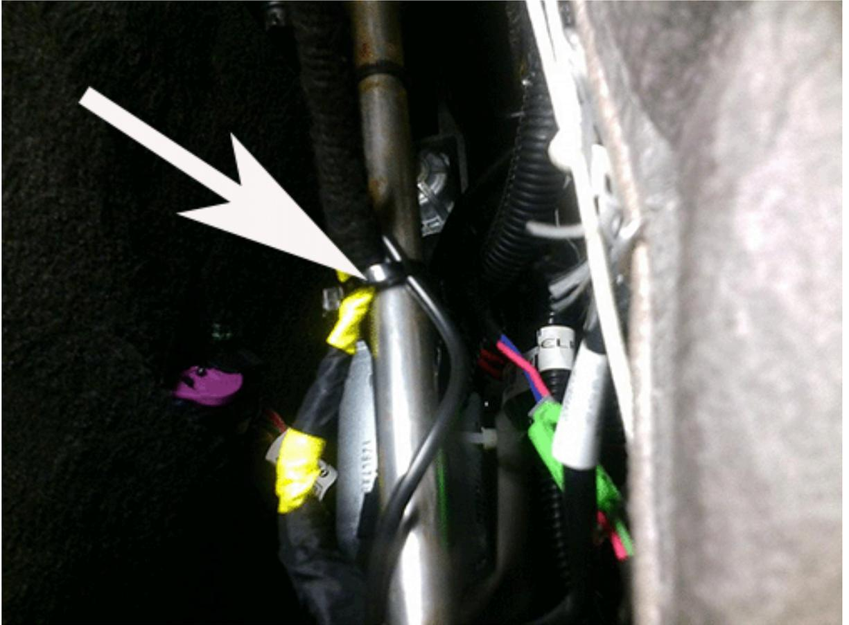
1. Install a wire tie, securing the harness to the seat in the original location. Ensure the wire tie is located on the body side of the wire splice.
