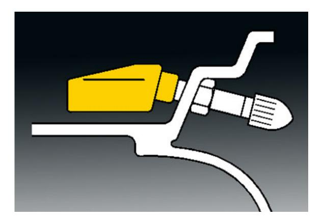
If the tire machine's bead breaking fixture is positioned too close to the TPM sensor, or pressed down directly on top of it, it may contact the sensor as the tire bead breaks away from the wheel rim. This can damage the TPM sensor and require the sensor to be replaced.
