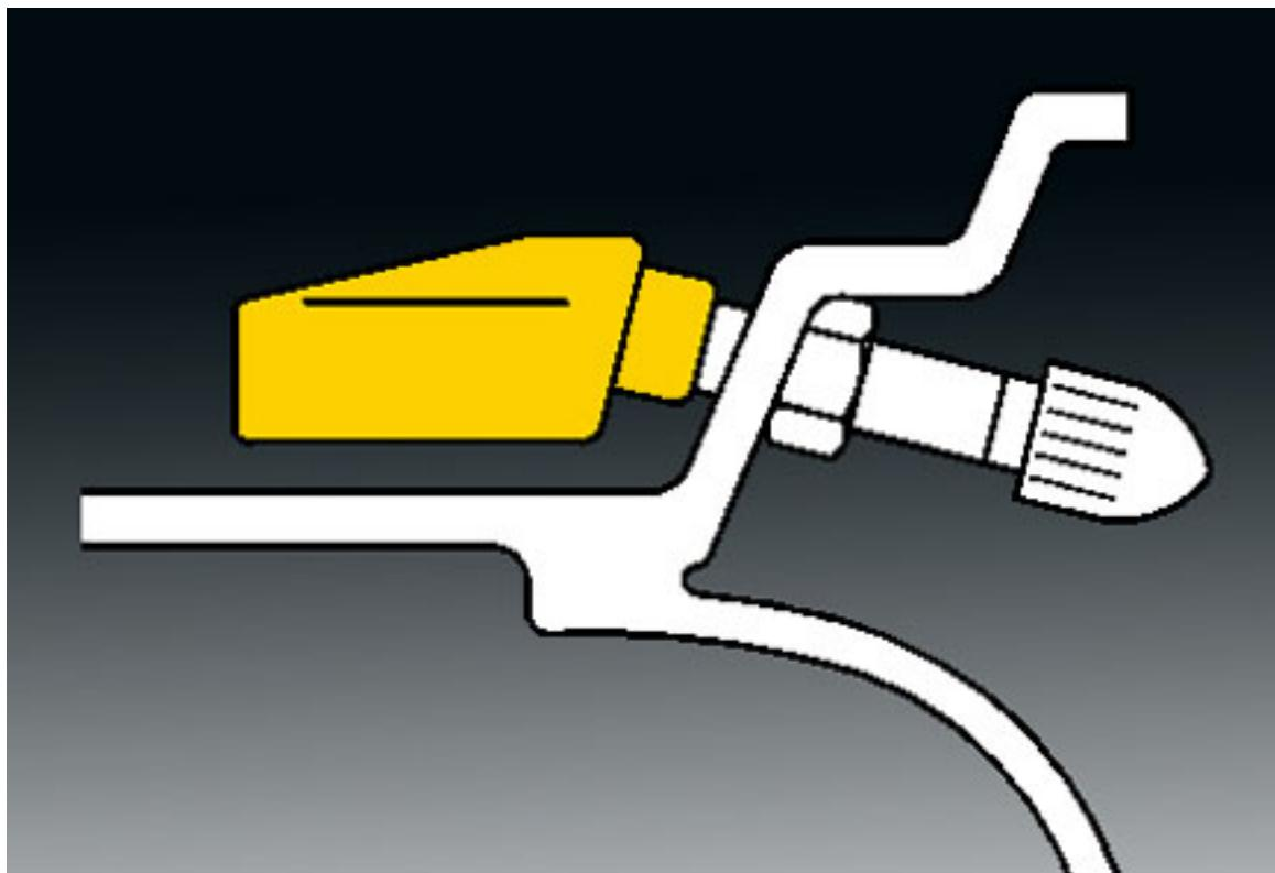
If the tire machine's bead breaking fixture is positioned too close to the TPM sensor, or pressed down directly on top of it, it may contact the sensor as the tire bead breaks away from the wheel rim. This can damage the TPM sensor and require the sensor to be replaced.
