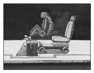
Get it up to speed. Then stop the vehicle. The rider doesn't stop.  $% \label{eq:condition}%$
