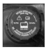
Then replace the pressure cap. Be sure the cap is fully installed.
