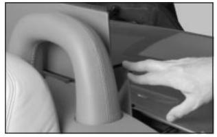
12. Manually move the front tonneau to the open position. Once the front tonneau is open, fold the side wings in by gently pressing them in. Do not force the wings. If they are hard to move, make sure the front tonneau is open all the way.
