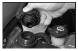
2. Then keep turning the cap and remove it.
