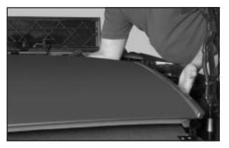
15. Hold the top in the front and side and lift the top out of the stored position.
