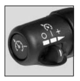
Some of the ACC controls are located on the end of the multifunction lever.
