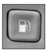
The fuel door release button is located on the left side of the instrument panel.
