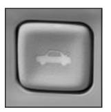
The trunk lock release button is located to the left of the steering wheel on the instrument panel. Press the button to open the trunk. To use this feature, your vehicle must be in PARK (P) or NEUTRAL (N) and the valet lockout switch must be off.
