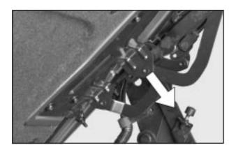
6. Pull both sides of the rear tonneau over-center link down to unlock the linkage.
