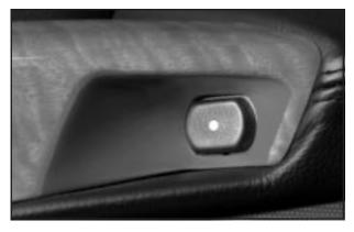
To open a door from the inside, press the button in front of the door handle and push the door open.
