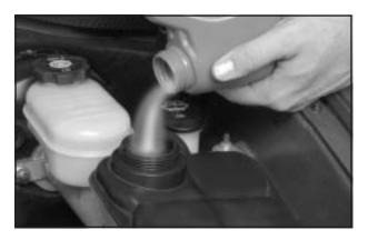
Then fill the coolant surge tank with the proper mixture to the full cold fill mark on the front of the coolant surge tank.
