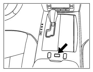
The AIR BAG OFF light on the center console will come on to let you know that the passenger's air bags are off. The passenger's air bags will remain off until you turn them back on again, and the AIR BAG OFF light will stay on to remind you that the air bags are off.
