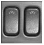
The power window switches are located on each door near the armrest.
