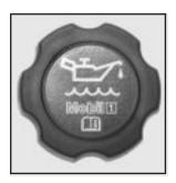
See Engine Compartment Overview on page 5-12 for the location of the engine oil fill cap. Be sure to add enough oil to put the level somewhere in the proper operating range. Push the dipstick all the way back in when you are through.
