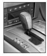
Move the shift lever into PARK (P) by pushing the lever all the way toward the front of the vehicle.
