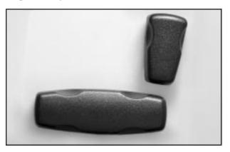
The eight-way power seat controls are located on the outboard sides of both the driver's and the passenger's seats.
