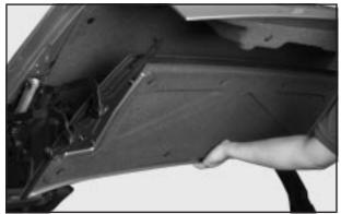
Move the rear tonneau rearward and up to the stored position. Pull from the center of the tonneau to keep pressure even. The rubber bumper on each corner will fit against the underside of the trunk decklid.
