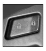
The power door lock switches are located on the door panels near the windows.
