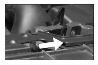
Then go to the front of the vehicle and find the secondary hood release lever. The lever is located under the hood near the center of the vehicle. Move the release lever to the right and raise the hood.
