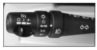
The exterior lamp control is located to the left of the steering wheel on the multifunction lever.
