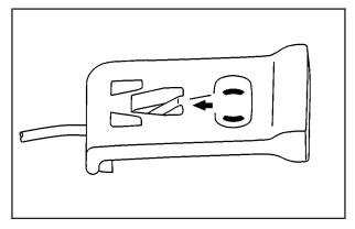
If you are outside the vehicle, there is a door release tab in the trunk. The tab is located behind a panel on the driver's side of the trunk. Pull the handle to unlock and unlatch the driver's door. See *Trunk on page 2-11* for information on opening the trunk during a loss of power.
