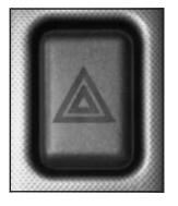
The hazard warning flasher button is located on the instrument panel above the navigation system.
