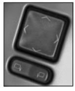
The power mirror control is on the driver's door armrest and controls the driver's side and passenger's side mirrors.
