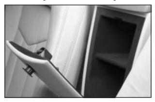
There is also an upright center console storage area between the seatbacks. To open the storage area, press and release the button near the top so it extends out. Then, turn the button in either direction to unlatch the lid and pull the console lid down. After you close the lid, press the release button back in.
