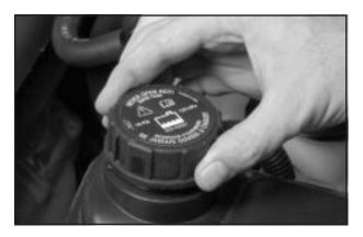
Park the vehicle on a level surface. You can remove the coolant surge tank pressure cap when the cooling system, including the coolant surge tank pressure cap and upper radiator hose, is no longer hot. Turn the pressure cap slowly counterclockwise (left).
