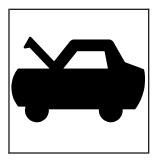
1. Pull the lever with this symbol on it. It is located on the lower left side of the instrument panel.
