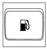
The fuel door release button is located on the left side of the instrument panel. The button only works when the vehicle is in PARK (P) or NEUTRAL (N) and the valet lockout button is in OFF. To remove the fuel cap, turn it slowly counterclockwise. The fuel cap has a spring in it; if the cap is released too soon, it will spring back to the right.
