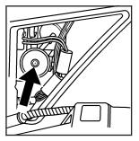
8. Turn the vertical aiming screw until the headlamp beam is aimed to the horizontal tape line. 9. The top edge of the cut-off should be positioned at the bottom edge of the horizontal tape line.
