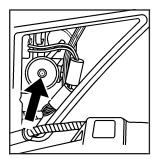
The headlamp aiming device is under the hood near the headlamps.
