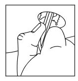
While holding the rear of the top down, insert the wrench into the bolt in the plug opening in the headliner.
